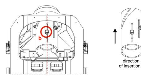
To take advantage of the maximum extension of the lens, position the knobs at the ends, loosening them and fixing them once the position has been found, as in Fig. 3.
